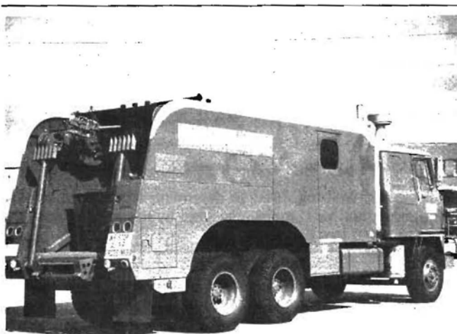
Trucks such as this contain logging equipment used to run electric logs, or other logs, on oil, gas, and geothermal wells.
