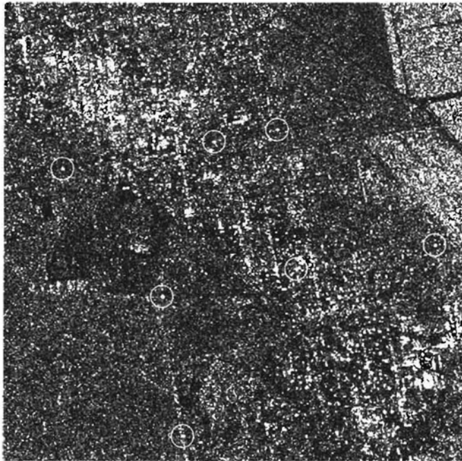
Figure 2. The RADARSAT-1 SAR image from February 25, 2001 showing the locations of the radar reflectors in the North Belridge oil fields.
