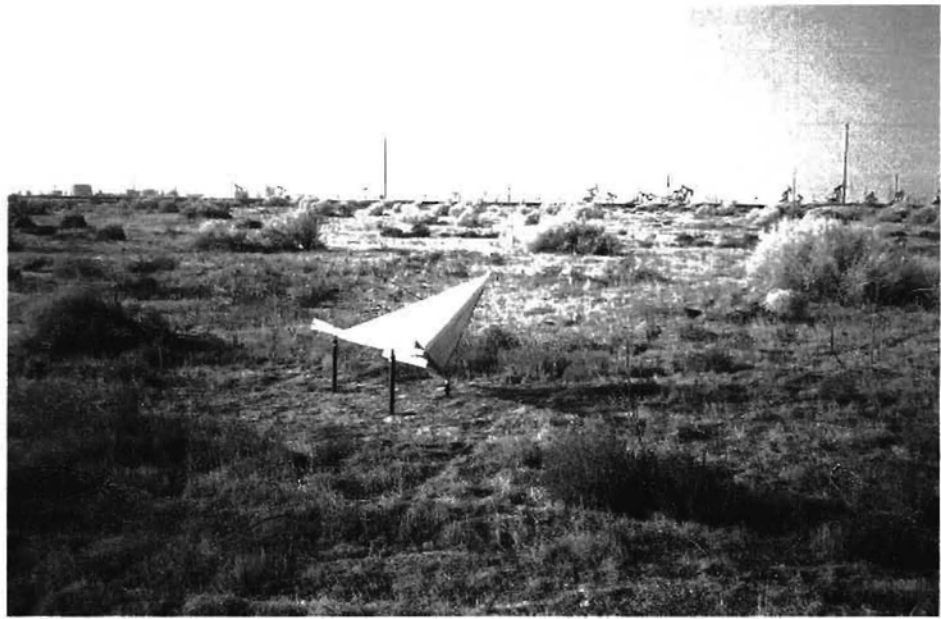
Figure 3. Example radar reflector installed in Belridge.
